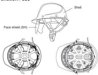
For with polyfoam shock absorbing liner
