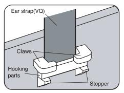
Install in 4 places, and be sure to check that both ends of the hooking part are between the claw and the stopper.
